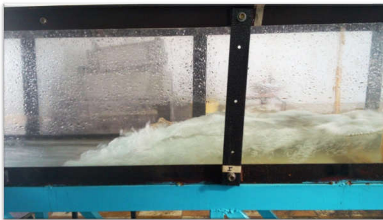
Figure (3) Hydraulic jump with adverse slope ( Q=15L/s , Fr_1= 5.74 and s=0.0043 )
