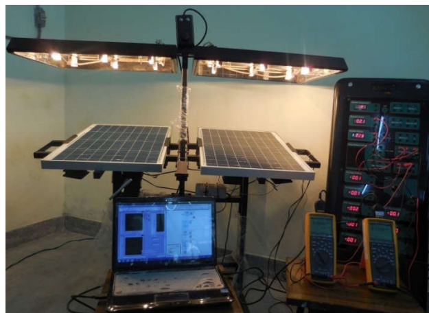
Figure 1: The constructed PV system experimental set up
