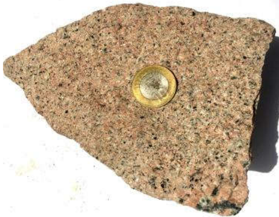
Photograph 7: Showing the Fine grained, equigranular variety of granite (Sample JB-5).
