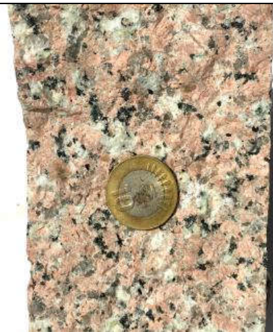
Photograph 8: Showing the Coarse grained, equigranular variety of granite (Sample JB-6).
