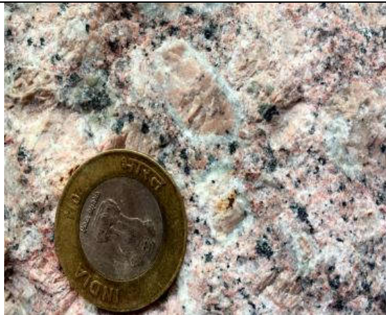
Photograph 9: Showing the inequigranular texture with Rapakivi structure (Sample JB-9).
