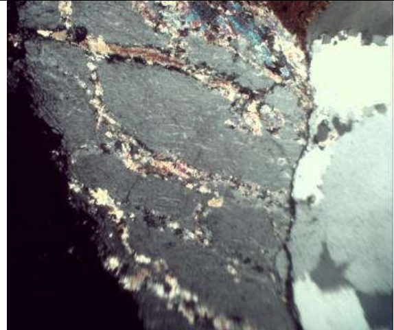
Photograph 14: Showing the alteration to sericite in potash feldspar (Sample JB-22)
