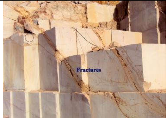
Photograph 6: Large scale fractures in the granites causing difficulty in block formation
