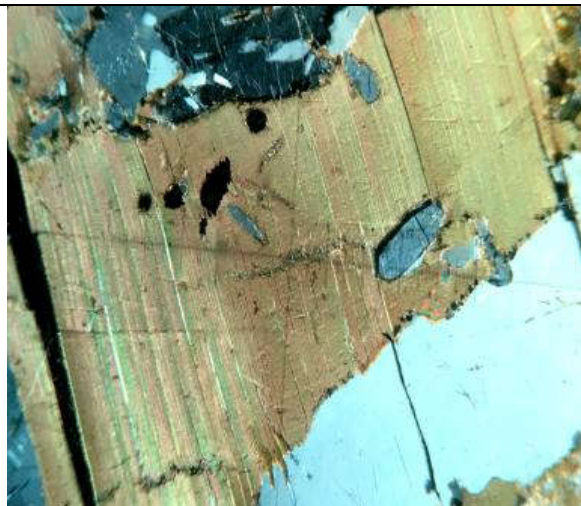
Photograph 17 : Inclusion of apatite and quartz within the biotite grain (Sample JB-14)
