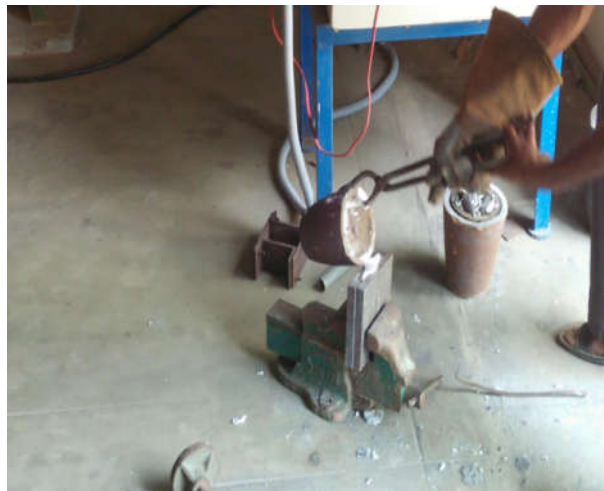
Figure.(b) Pouring metal into the mould cavity
