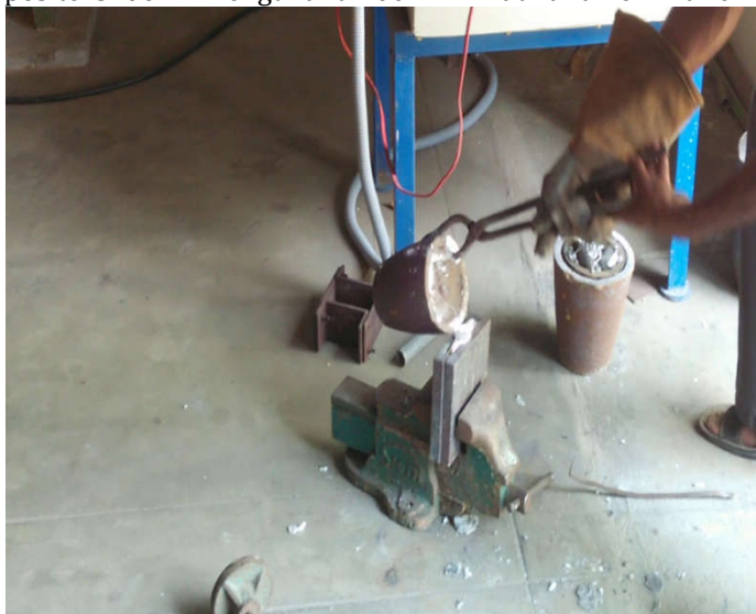
Figure.2. Pouring metal into the mould cavity
