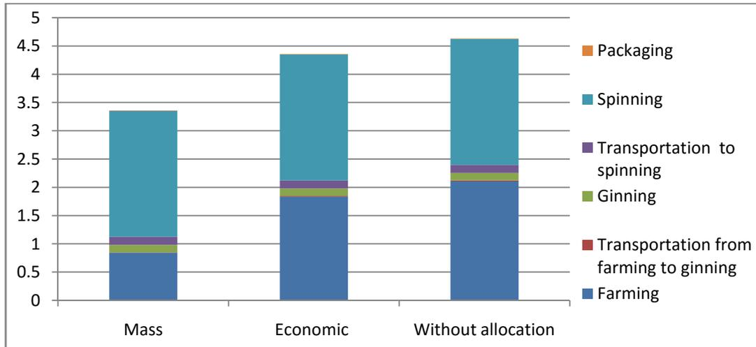
**Figure 6: Distribution of electricity in various stages of life cycle stages of cotton yarn**
