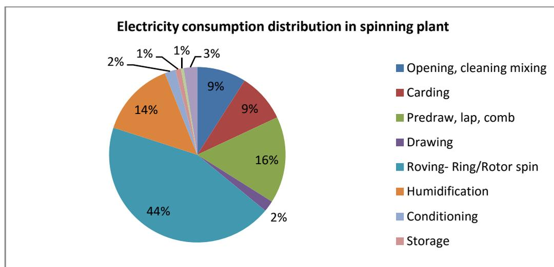
**Figure 5: Distribution of electricity emissions in various stages of spinning**
