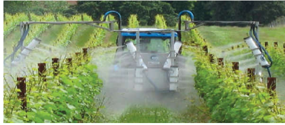
Fig. 2. Application of chemicals using Electrostatic spraying
