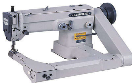
Fig 6: JUMBRO sewing machine: Suitable for medium-heavy artificial leather materials
