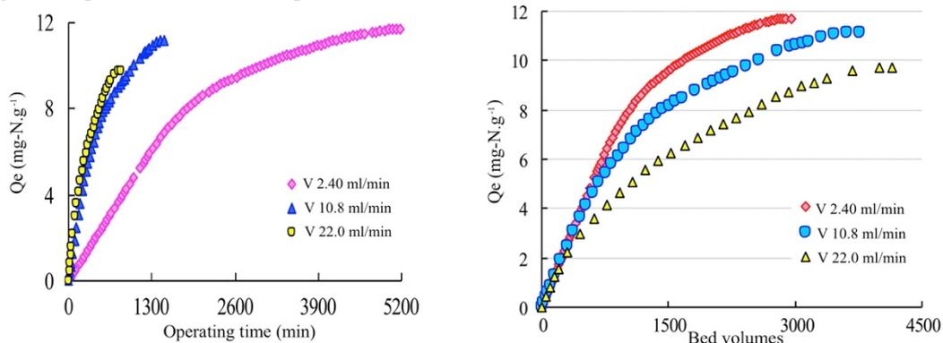
**Figure 3.** Results of  $\text{NH}_4^+$  removal by zeolite in columns
