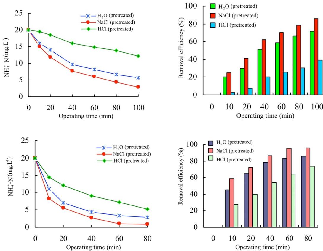
Figure 1 Effects of pretreatment on NH<sub>4</sub><sup>+</sup> removal by zeolite: (a)- (b)Clinoptilolite, and (c)-(d)Mordenite.
