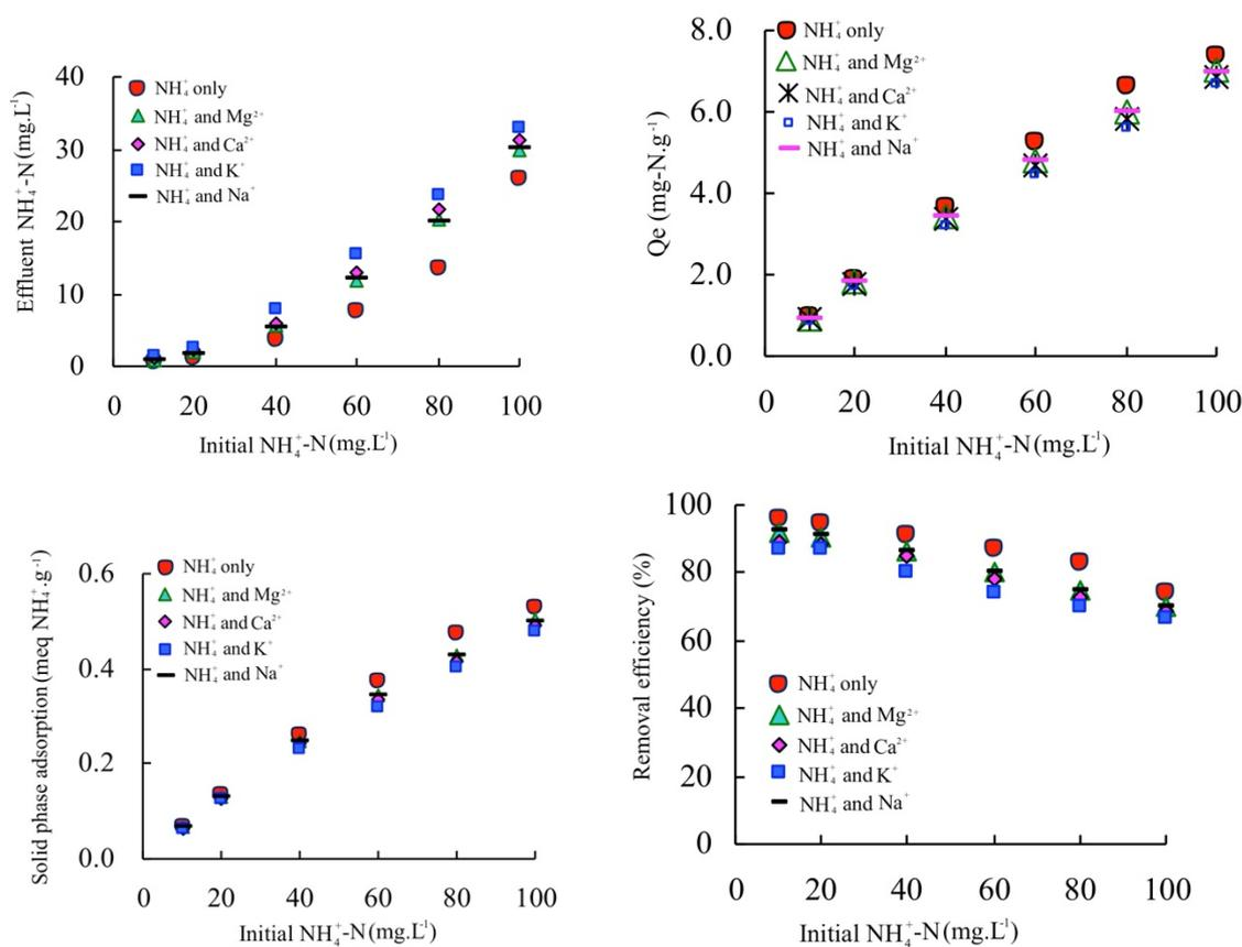
**Figure 4.** Ammonium exchange isotherms and effects of individual cation on the exchange of  $\text{NH}_4^+$  uptake by zeolite.
