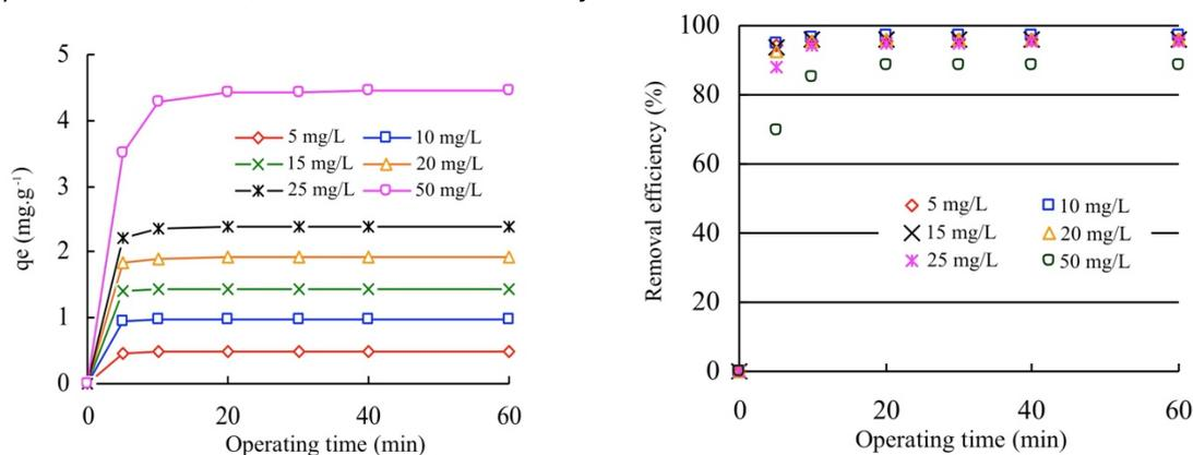
**Figure 2** Effect of contact time and initial conc. on the exchange of  $\text{NH}_4^+$  onto clinoptilolite (T,  $20^\circ\text{C}$ )
