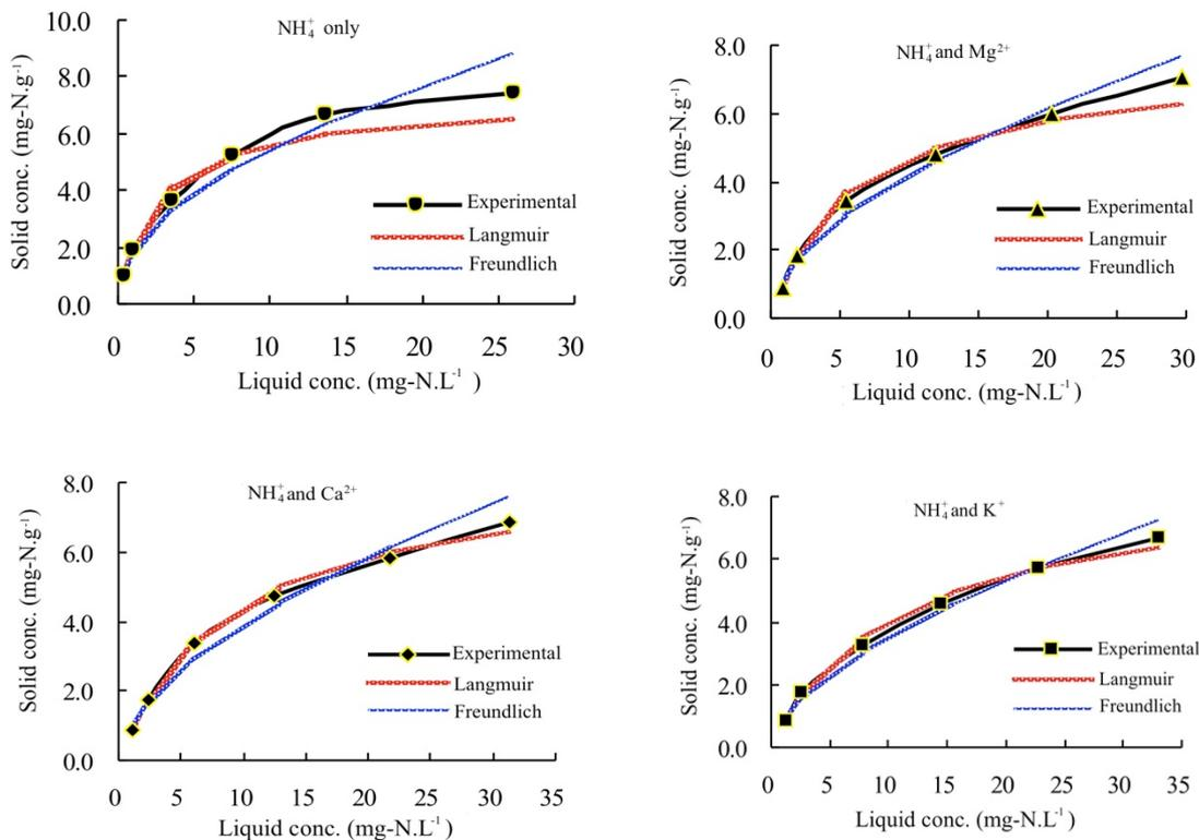
**Figure 5.** Equilibrium isotherm data for  $\text{NH}_4^+$  uptake onto clinoptilolite fitted to the Langmuir and the Freundlich uptake models under the condition of  $\text{NH}_4^+$  only, and in the presence of individual  $\text{Mg}^{2+}$ ,  $\text{Ca}^{2+}$ ,  $\text{K}^+$  ion.
