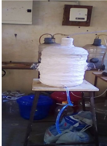
Figure 1. Experimental set up of aerobic batch reactor
