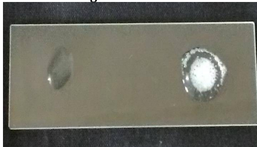
Figure 8. catalase test- Positive result in air bubbles formation
