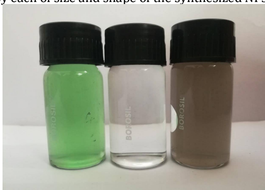
Figure 2. AgNPs changes color from green to brown after the addition of silver nitrate solution
