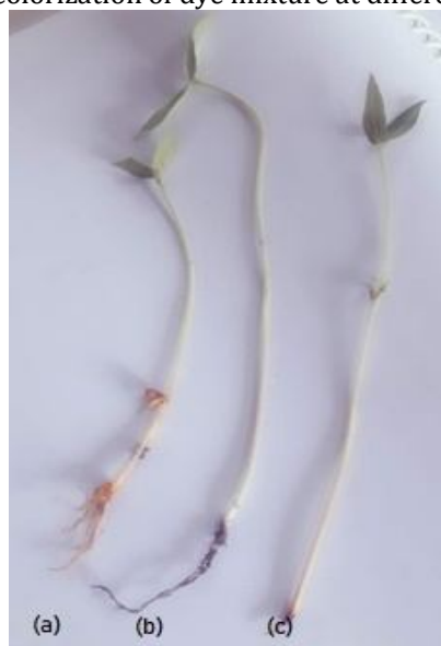
Figure 3. Phytotoxicity studies on seeds of Green gram watered with (a) Distilled water (b) Decolorized solution (c) Dye solution
