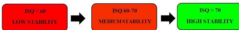
Figure 8: Significance of implant stability quotient values as displayed through the Osstell mentor
