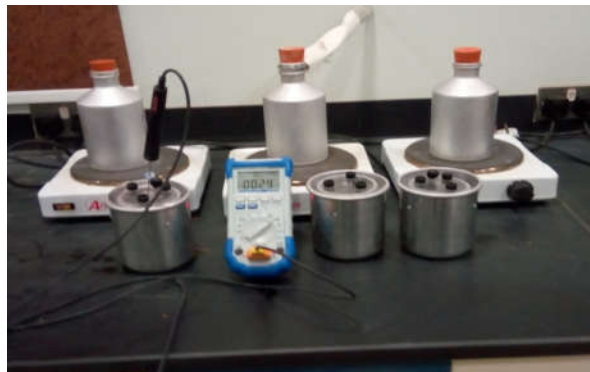
Figure 1: Shows a set of Calorimeter using to measure the Specific Heat of the samples meats
