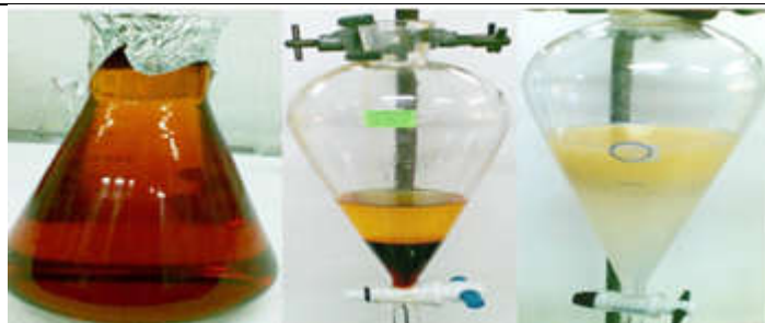
Fig. 1. A) Filtered waste sunflower cooking oil, B) Phase separation, upper is biodiesel and C) Formation of emulsion
