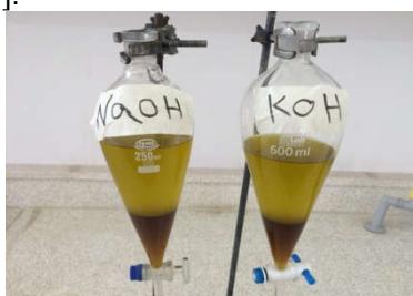
Figure 1: production of biodiesel and deposition of glycerin
