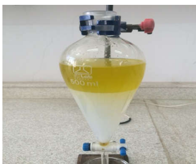
Figure 3: leaching the produced biodiesel
