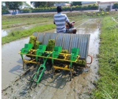
Fig1: Urea briquette applicator with self-propelled rice transplanter
