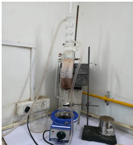
Figure 2: Preparation of Extract by Soxhlet Method
