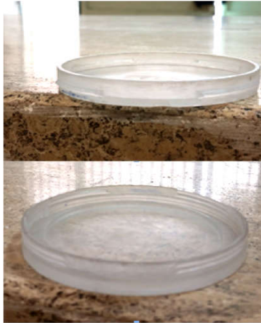
Figure 1: The designed Petri dish. Upper part: the lid, underneath part: the container with caulking loop.
