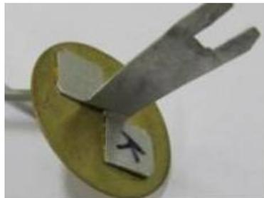
**Figure 1: Piezo based Cross Type sensor for Dental implant stability Measurement**
