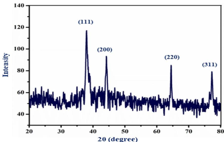
**Fig. 3 XRD illustration of *Gomphrena celosioides* mediated Ag NPs**
