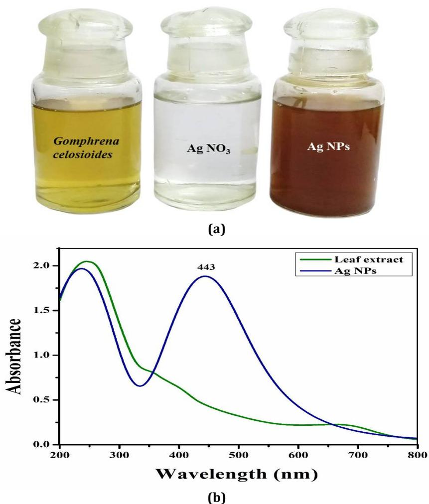
Fig. 1 (a) Colour intensity of *Gomphrena celosioides* aqueous extract and Ag NPs, (b) UV-visible spectrum of Ag NPs after 180 min from the reaction.
