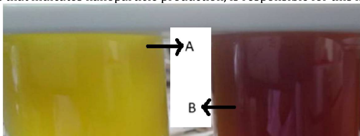
Figure 4: Biosynthesis of AgNPs Using Leaf Extract. Where leaf filtrate: A = Prior to the addition of 10 mM \text{AgNO}_3 solution; B = After treatment with 10 mM \text{AgNO}_3 solution
