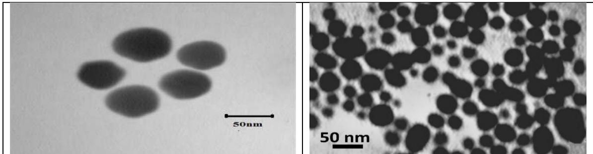
Fig. 2. Transmission electron microscope images of synthesized silver nanoparticles with different magnifications.
