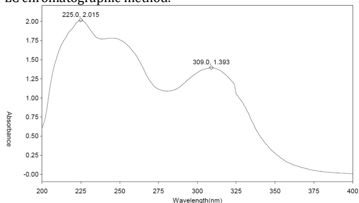
Fig. 2: UV-VIS spectrum of CHLORTHALIDONE (225 nm)
