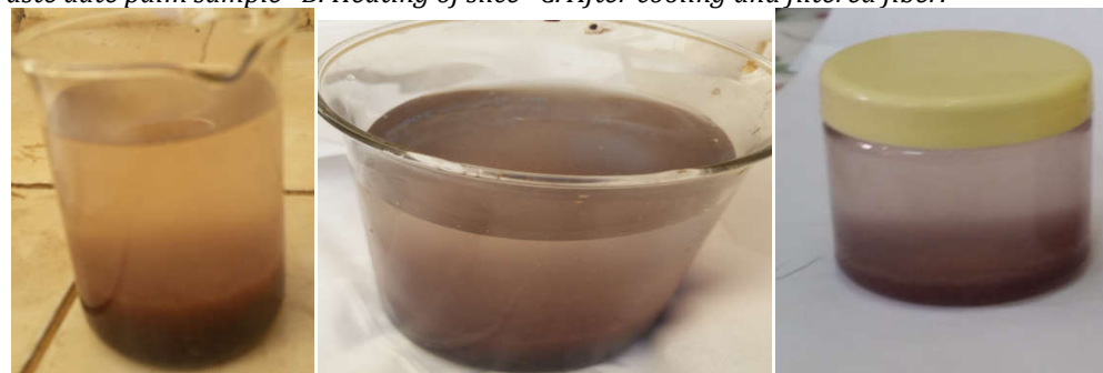
D. Acid hydrolysis and nanocellulose E. Nanocellulose mixture F. Nanocellulose
