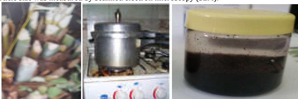
A. Waste date palm sample B. Heating of slice C. After cooling and filtered fiber.
