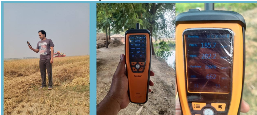
Figure 4. Ambient air quality in respect of Particulate Matters (PM) of Murulia village was measured through Temtop M2000C Air Quality Monitor
