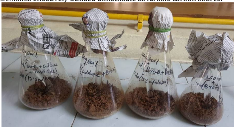
Figure 6: Experimental setup for CO 2 evolution
