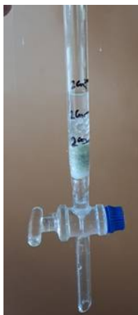
Figure 9: Biofilter setup using Pseudomonas biofilms
