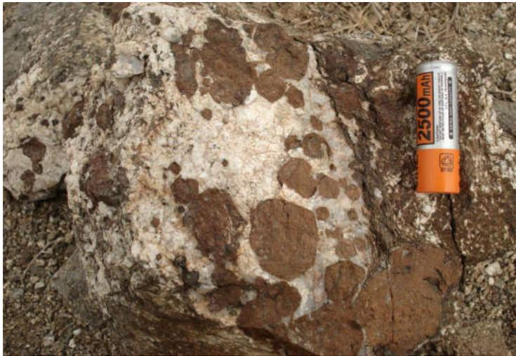
Fig.3. large crystals of garnet (brown) in quartz veins of Dehchah. Garnet frequency above 35 percent in some areas that could be of economic value
