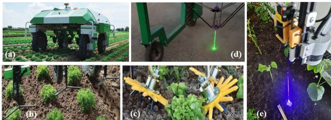
Figure 4. (a-c) Mechanical weeding robot; (d,e) Thermal/Laser Weeding robots
