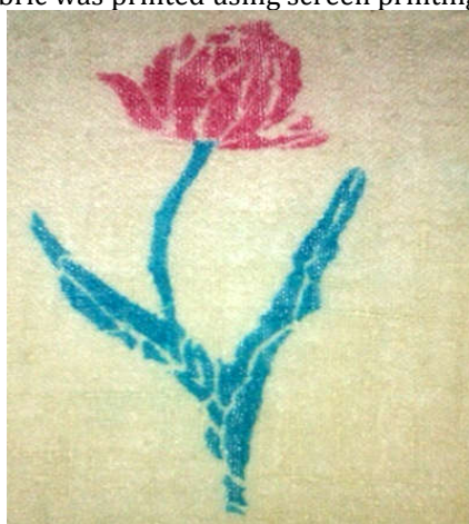
Plate 1: Screen printing using reactive red 198 (flower) and reactive blue 21 (stem and leaves) dye
