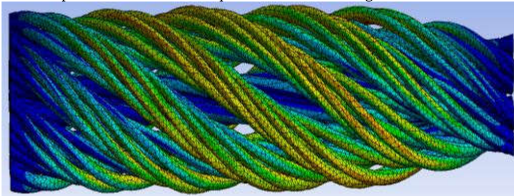
Figure 7 Stress distribution in wire rope 2
