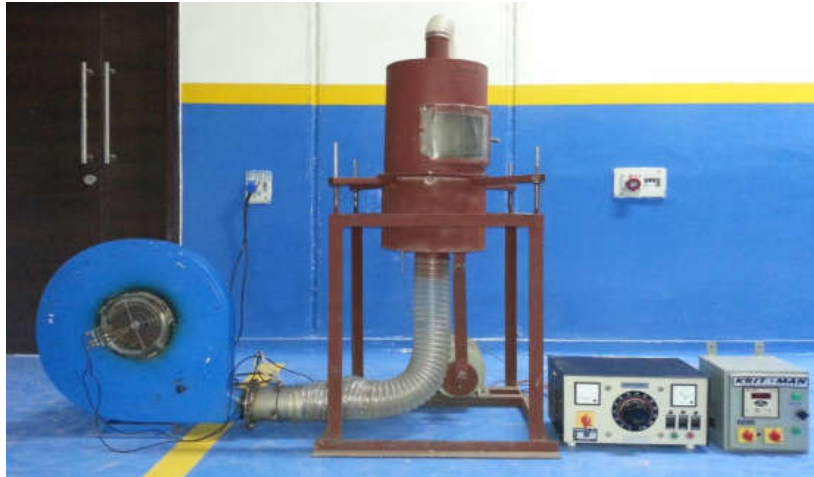
Fig. 1: Experimental setup of Vibro-Fluidized Bed Dryer
