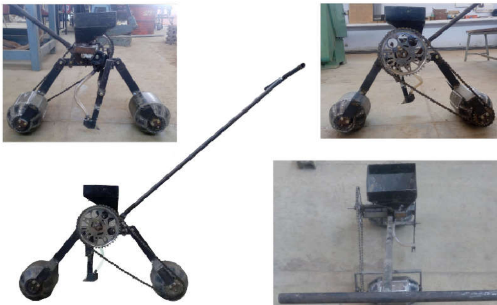
Fig. 5: The developed ridge vegetable planter
