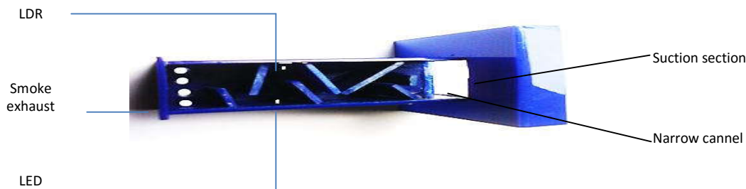
Figure 4: Smoke sensing system
